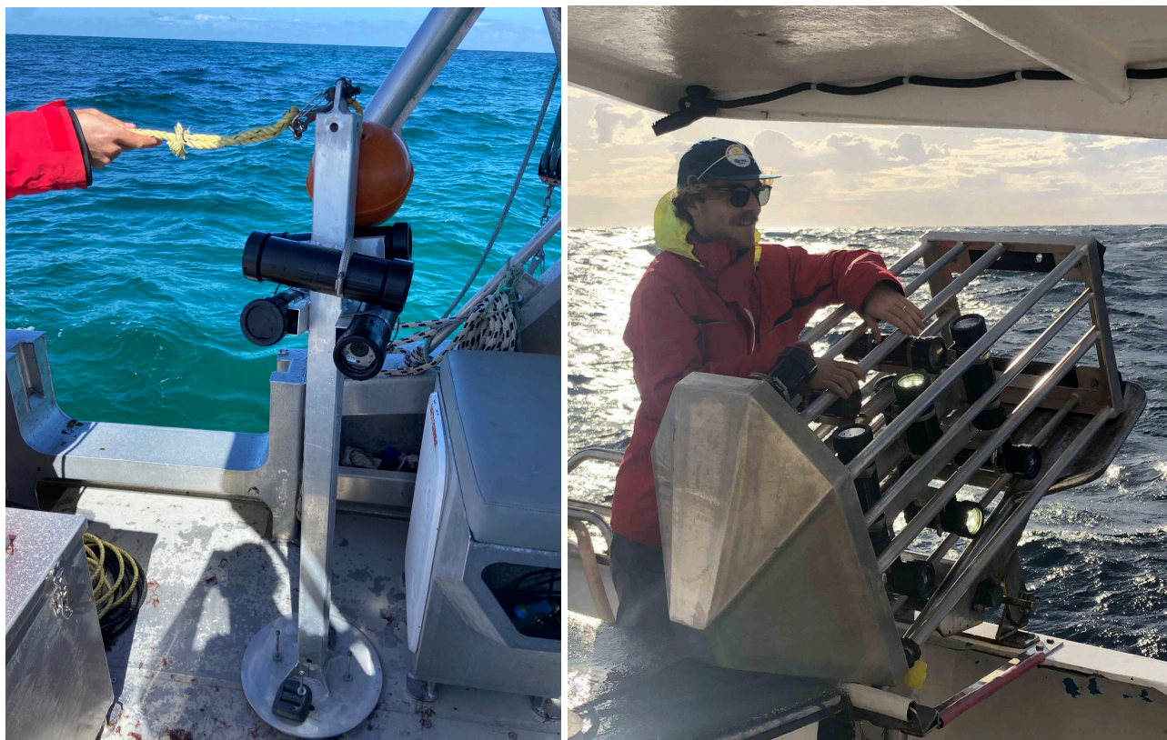
Figure 4. Lighter weight mono-configuration wide-field drop camera system being deployed by hand (left) and stereo-configuration wide-field drop camera system deployed from a commercial fishing vessel fitted with a ‘pot tipper’ (right).
